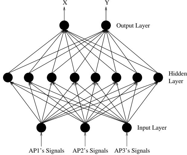
**Fig. 1.** An example of multi-layer perceptron configuration
